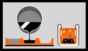
The liquid metal thus obtained is poured into sheets then undergoes a chemical and electrochemical treatment: the various baths and the <u>electrolysis</u> applied by the treatment company enable the separation of the different metals and alloys. This is "dealloying".
