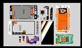
On arrival, the smartphones are taken apart: on one side the plastic shells, which are sent to specialists of this material. On the other, the screens and electronic components that Morphosis will recycle.
